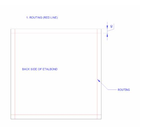
The first step for making an etalbond® cassette is cutting the panel in shape. In the example shown above, the aim is to make a cassette of dimensions 800mmx800mm and 40mm depth. The edges of the cassette will be folded 40mm. Therefore, the first step is to cut a piece that is 40mm + 40mm wider than the size we wish to create. In the example it will be (800+40+40)=880, so the piece we cut will be 880x880mm.
