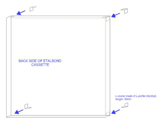
In order to stiffen the cassette, it is important to fix aluminium L-profiles inside the corners of the cassette. For the example shown above, a 30x30x2 aluminium L-profile is used. By cutting small pieces of this profile (in 30mm lenght) we create small angles that can be placed in the 4 corners as shown in the drawing above. Before placing the corners it would be better to put silicone in the corner in order to waterproof the cut edges of the cassette.
