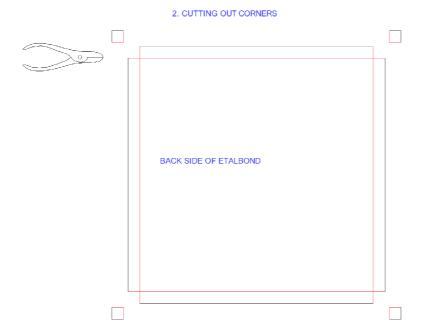
The corners that are created by the routing must be cut out, in order to allow us to fold the edges of etalbond®.
