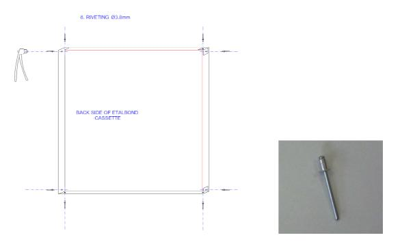
In the holes we drilled we fix rivets of 4.8mm (or 3.8mm) diameter.
