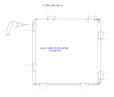
Holding the corners in place, we drill 2 or 3 holes of 5mm diameter.
