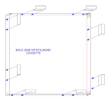
Using the aluminium L-profile of 30x30, we cut again pieces of 100mm length and place them with one "leg" inside the cassette.
