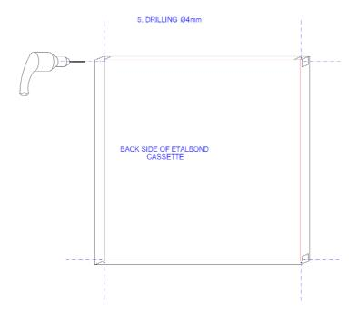
Holding the L-corners in place we use a drill of diameter 5mm (or 4mm) to create holes through both etalbond® and the L-corners according to the blue dotted lines shown in the drawing above.
