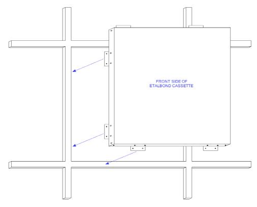
On the building we create a grid of galvanized hollow steel sections. A typical steel section that can be used is 40x20mm with thickness 1,5mm - 2mm. Then we place the cassette as shown in the drawing above.
